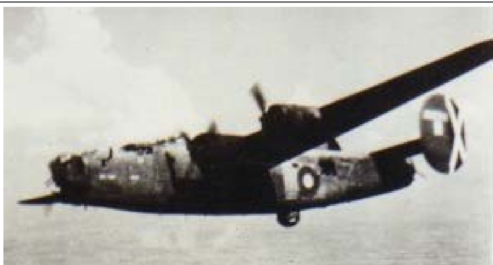
The C/O's Liberator BV1 (See the Wing Commander's markings under the cockpit) this aircraft has no bombing missions and is a new delivery to 356 Squadron. It is a very early type Liberator, note the extended pitot-tube which was only on the earlier delivered RAF Liberators. The serial is EV860 and the code 'Z'
