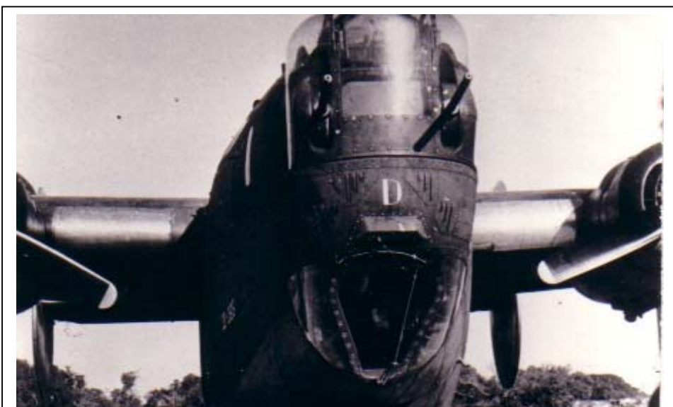
Close-up of the front turret and the bomb aimer's window and the code letter 'D'. The aircraft is KH284 of 99 Squadron
